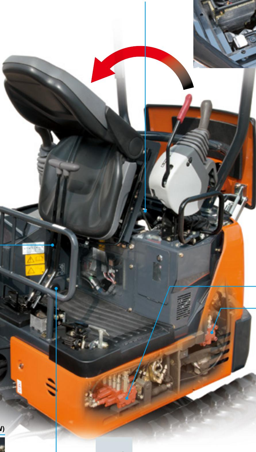
With the 2-way selector valve, the operator can effortlessly select the piping for the breaker or grapple.
