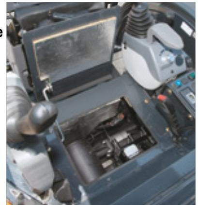
\*It is required to remove a plate from under the seat.
