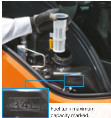
Fuel tank maximum capacity marked.
