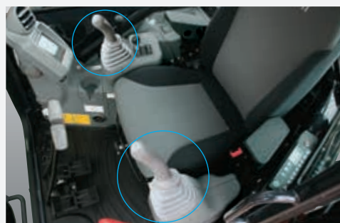
Control lever Shown equipped with cab, armrests, air conditioner, pedal and FM/AM radio as optional items.
