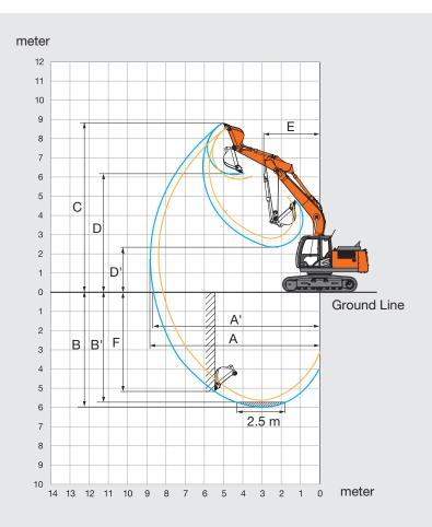
ZAXIS 160LC Arm length 2.22 m 2.58 m A Max. digging reach 8 520 8 870 A' Max. digging reach (on ground) 8 340 8 700 B Max. digging depth 5 620 5 980 B' Max. digging depth (2.5 m level) 5 340 5 740 C Max. cutting height 8 620 8 880 D Max. dumping height 5 940 6 170 2 750 D' Min. dumping height 2 380 E Min. swing radius 3 290 2 910 F Max. vertical wall digging depth 4 510 5 160
