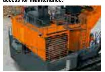
A walkway around the entire counterweight provides easy access to key rear areas. This means faster and safer inspection and maintenance.
