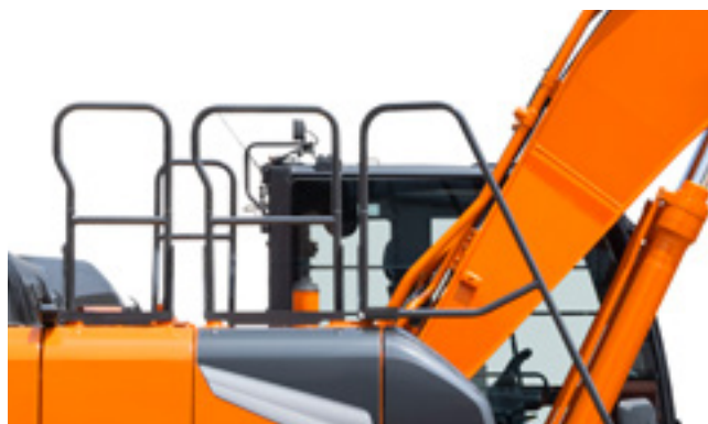
New hand rail on the ZX200-7 & ZX210LC-7 is retractable for easy transport.
