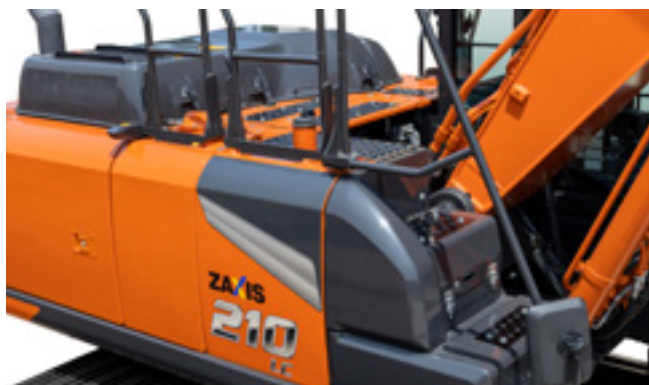
Wide steps on the ZX200-7 & ZX210LC-7 allow for easier maintenance.
