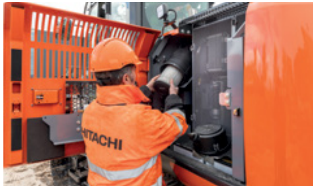
Filters and separator are conveniently located for ease of inspection and replacement.
