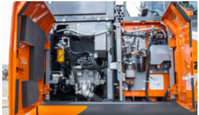
Filters and separator are conveniently located for ease of inspection and replacement.
