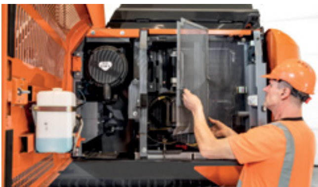
The air conditioner condenser can be opened for easy cleaning of the condenser and radiator located behind it.
