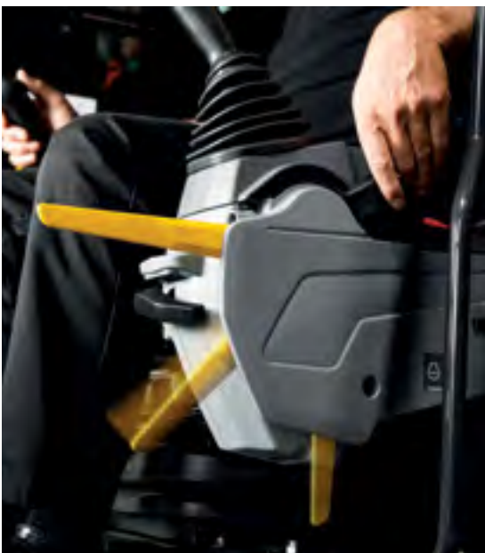
The pilot shutoff lever offers enhanced safety in the cab.
