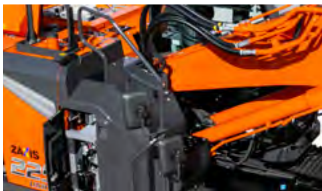
Wide steps on the ZX225US-7 & ZX225USLC-7 allow for easier maintenance.
