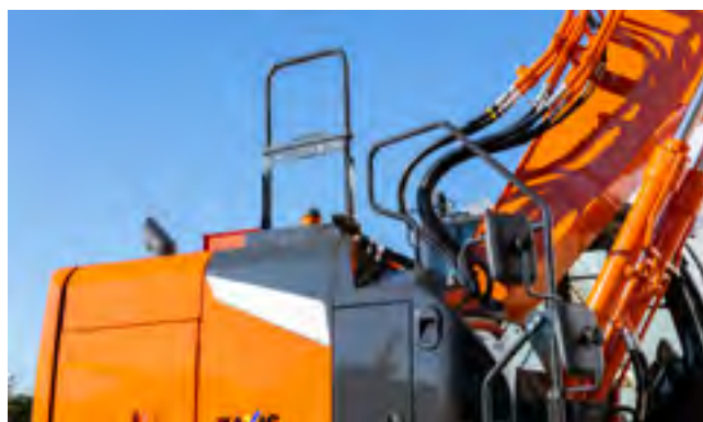
New hand rail on the ZX225US-7 & ZX225USLC-7 is retractable for easy transport.
