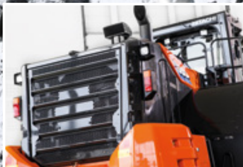
New rear grill protects radiator compartment.
