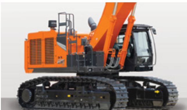
Access to the upper structure is easy via a new step.
