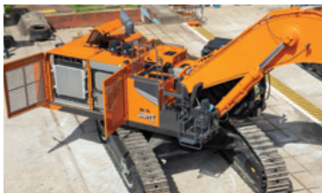
Components are conveniently accessible for daily maintenance.
