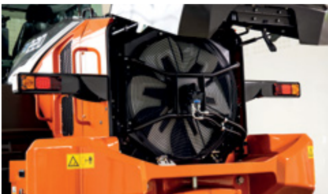
Intelligent fan operation system prevents radiators clogging.
