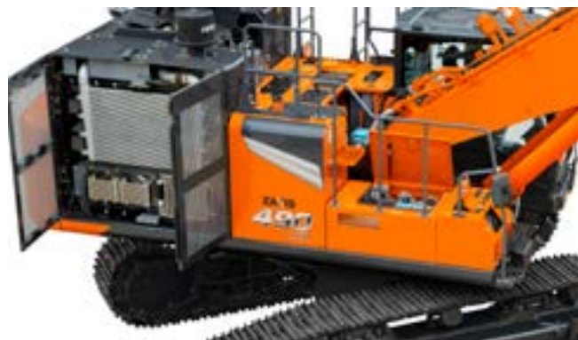
Maintenance is easy at ground level.
