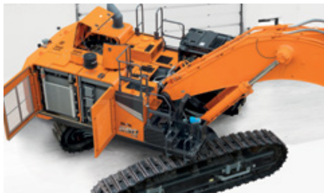
Components are conveniently accessible for daily maintenance.
