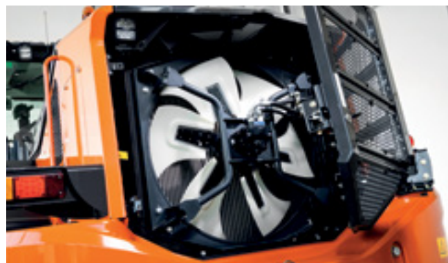
Intelligent fan operation system prevents radiators clogging.
