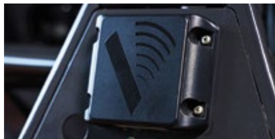
Rear obstacle detection system enhances safety on the job site.
