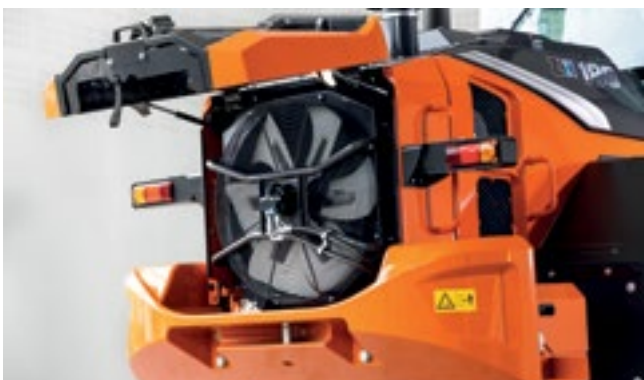
Intelligent fan operation system prevents radiators clogging.
