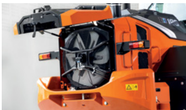
Intelligent fan operation system prevents radiators clogging.
