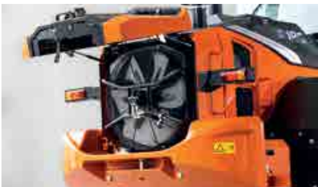
Intelligent fan operation system prevents radiators clogging.
