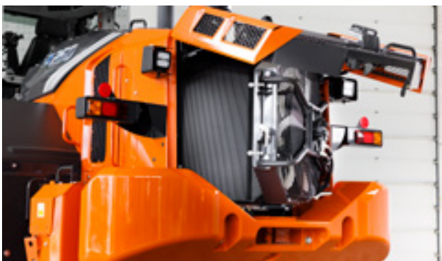
Intelligent fan operation system prevents radiators clogging.
