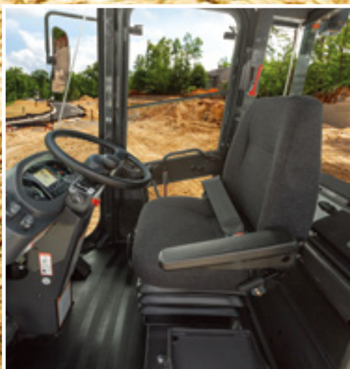
A standard suspension seat absorbs shock and vibration.
