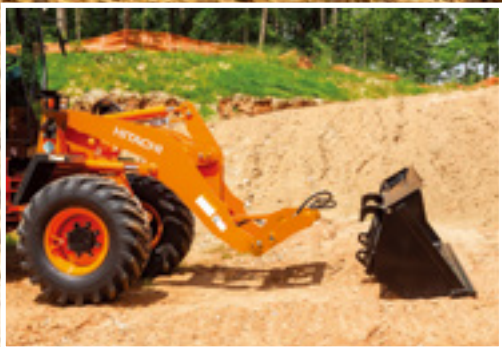
Optional pin-on type Quick Couple allows seamless transition (hydraulic for ZW80-SE).
