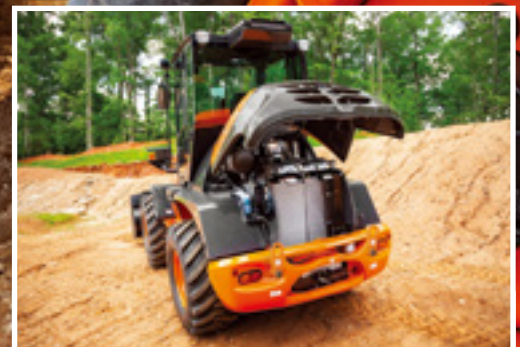
Easy access for maintenance from ground level.
