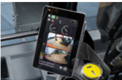
Low-reflective collar 8inch LCD monitor
