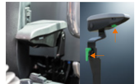
Toolless height and angle adjustable armrest
