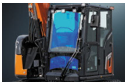
Shown equipped with additional counterweight and ambient LED lights, assist piping, pad crawler shoe (optional).
