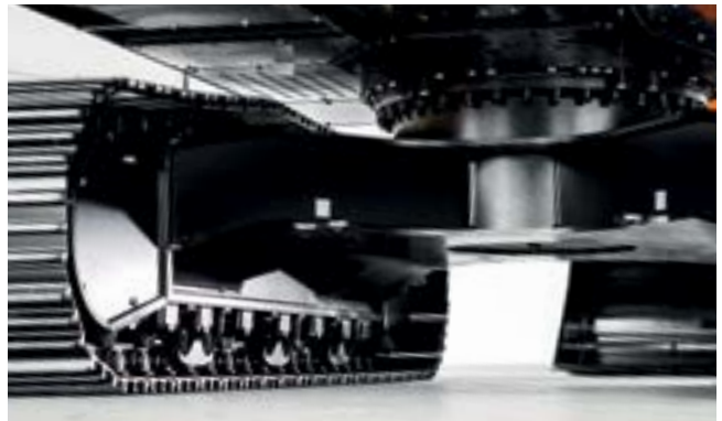
Strong X-beam, undercarriage and under covers enhance durability.
