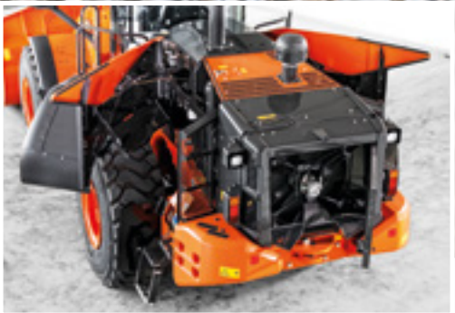
Covers open fully to give easy access for maintenance.
