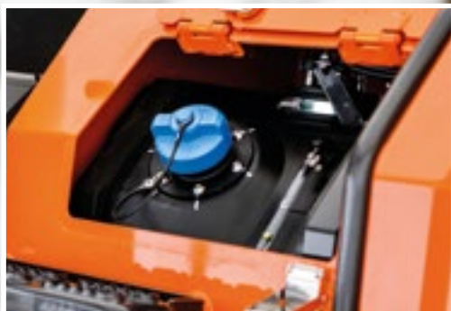
Urea is injected into the exhaust gas to reduce emissions.
