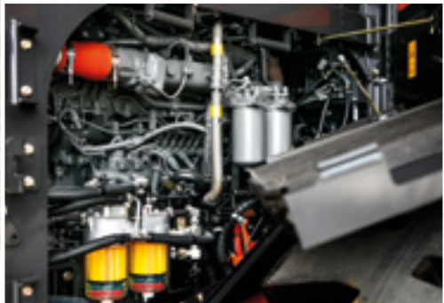
Stage IV engine reduces fuel consumption.
