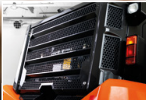
New rear grill protects radiator compartment.
