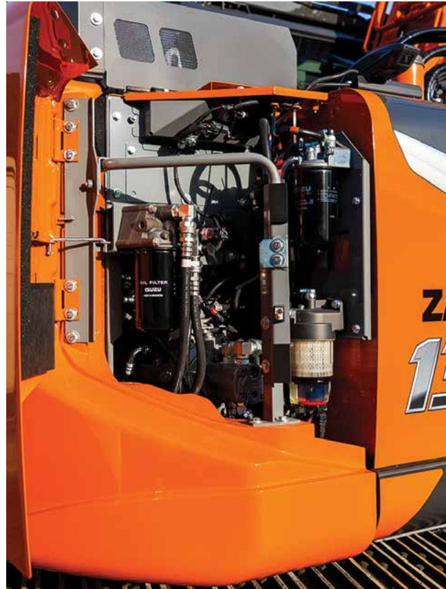
Filters and separator are conveniently located for ease of inspection and replacement.
