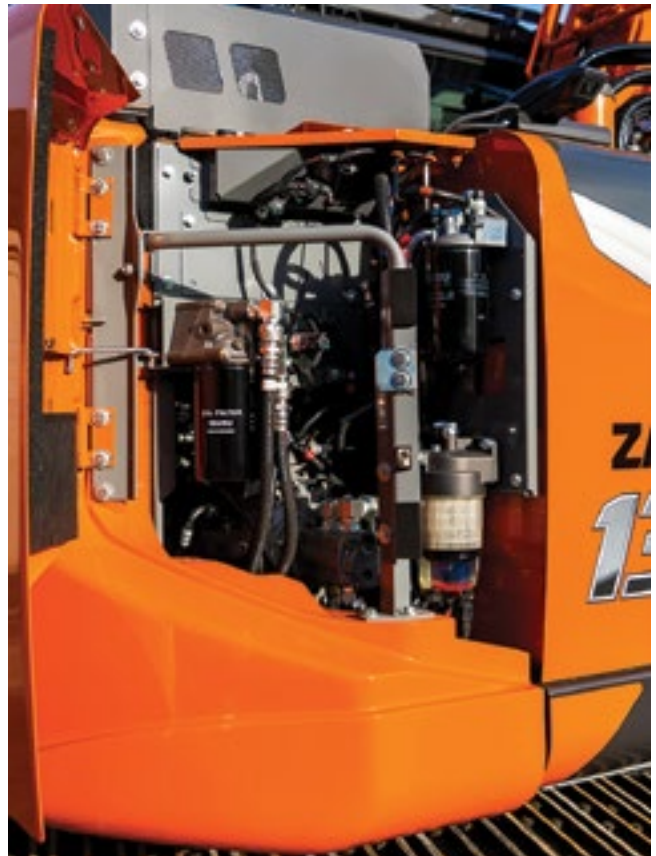
Filters and separator are conveniently located for ease of inspection and replacement.
