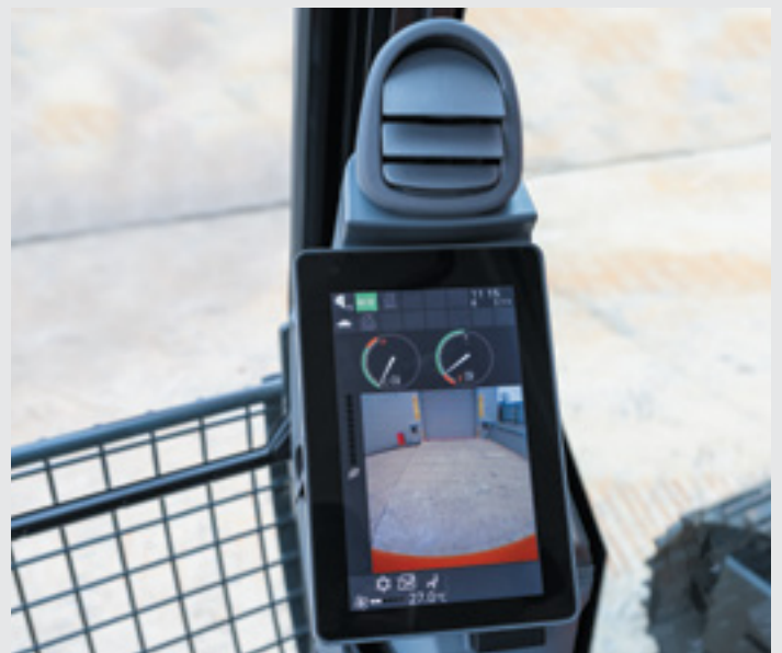
Low-reflective color 8" monitor, 42% larger display compared to ZX-5G series. Easier to view and navigate. Bluetooth® and optional USB power supply available.
