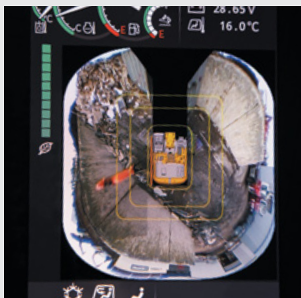
AERIAL ANGLE (Optional) 270-degree bird's eye-view camera system is available as an option.
