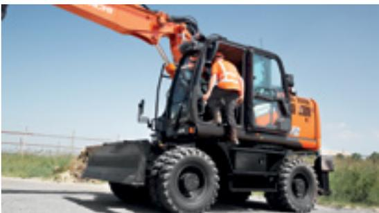
The lower first step makes entering the cab safer and easier.
