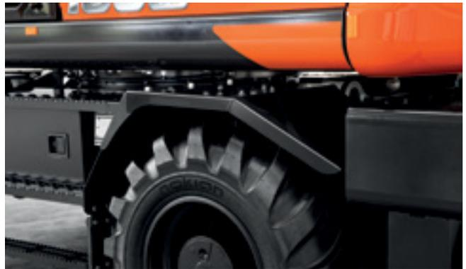
Fenders on the undercarriage protect the upper structure and lights from dirt, keeping the machine clean.
